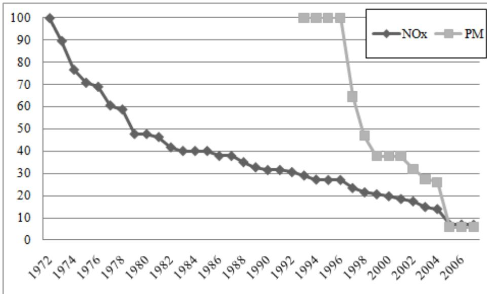
Note: The values are average because emission intensities are set by vehicle type. The standard values are set to 100. The standard value of NO<sub>x</sub> and PM is in 1972 and 1993, respectively.
